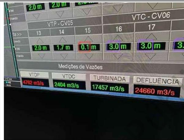
Photo 32: Power plant generating 2,469 MW (i.e. below capacity) while spilling 7,166 m<sup>3</sup>/s
