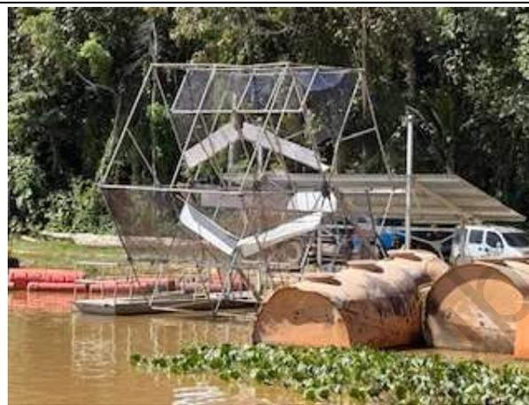
Photo 8: Experimental 'fish wheel' for fish monitoring at SAE port on reservoir
